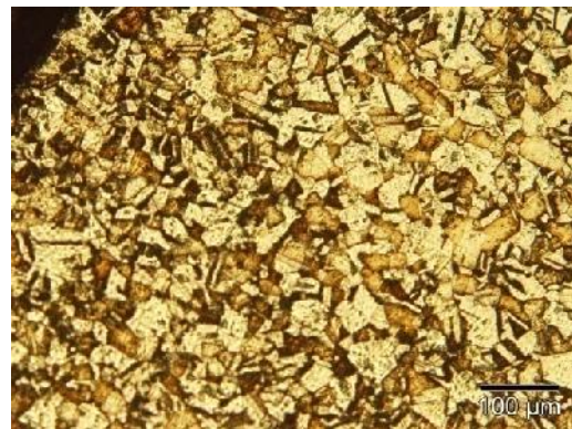
Fig-21 , Microstructure after final pillgaring outside tube
