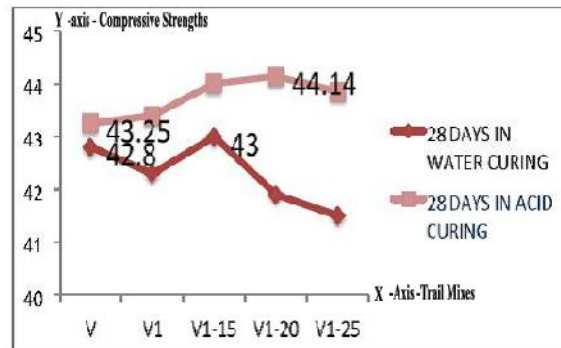
GRAPH 1: Variation of Compressive Strength at 28 Days with Replacement of Coconut Shells InCase Of Normal Curing and Acid Curing
