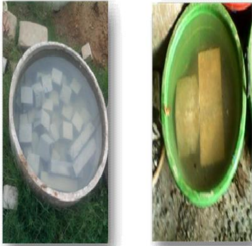
Fig. 4 1) curing in normal water 2) Curing of cubes in HCL Solution
