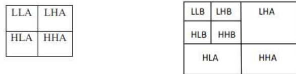
Figure 1: DWT showing its sub-band.
