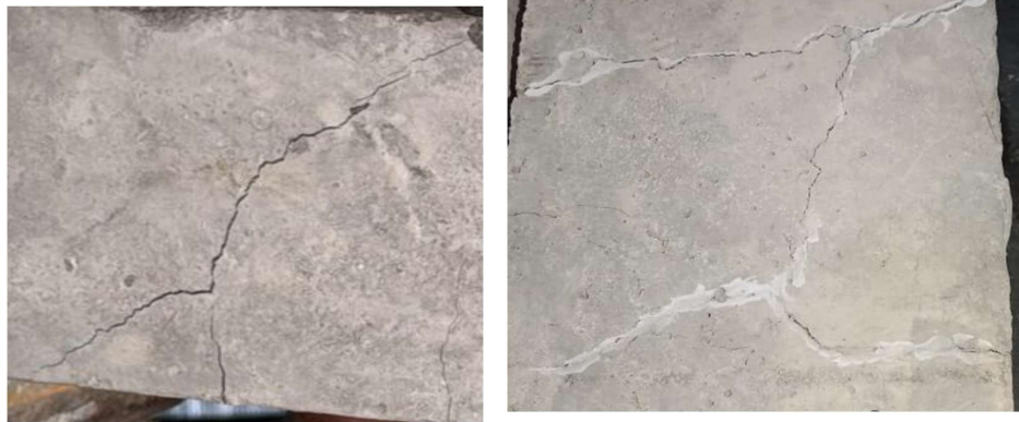
Fig.8 Visual inspection after 3 days of bacterial treatment
