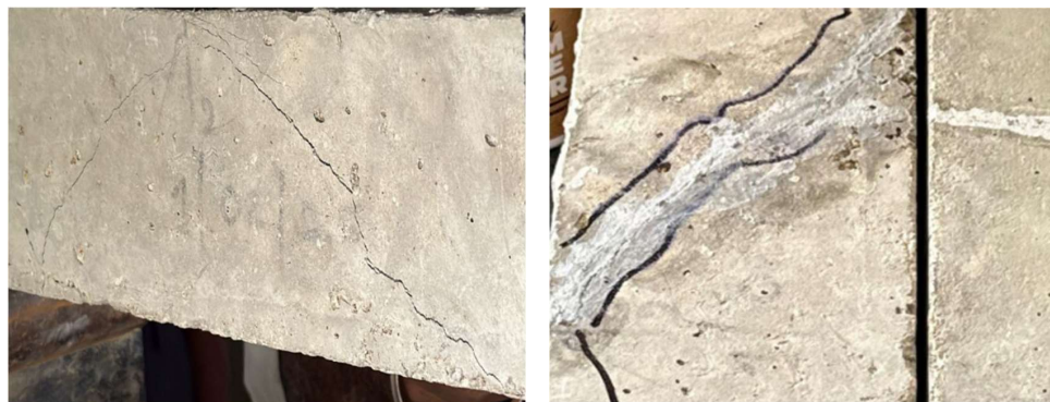
Fig.9 Visual inspection after 7 days of bacterial treatment
