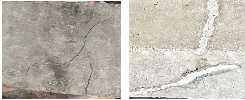
Fig.10 Visual inspection after 14 days of bacterial treatment
