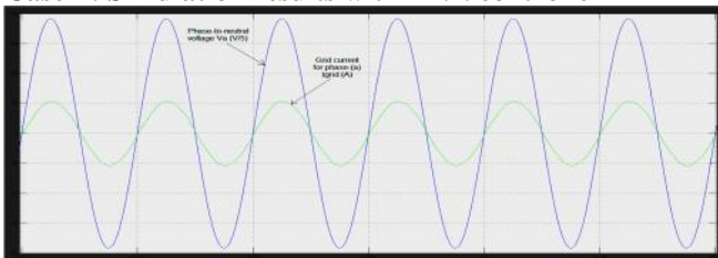
Fig.13 Phase-to-neutral voltage and grid current for phase-A with ANN controller
